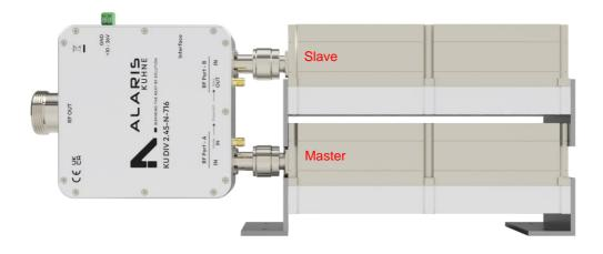
The generators are configured and labeled as master and slave before delivery. The master and slave must then be connected to the combiner with SMA cables according to the labeling on the combiner. In addition, for communication, the combiner must be connected to the two generators for the interface connector (I2C bus)
